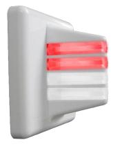
The **NC-DL-22-RW** is a stylish, exceptionally bright Nurse Call Dome Light and Controller all in one unit. It is the central tie point for the Patient Room, with wiring going to the Call Stations and to the Central Control Module. The Call stations are equipped with Momentary Switches that are monitored and latched in the Dome Light. The Call stations have Call Confirmation Indicators that display the same output as the Dome Light.
