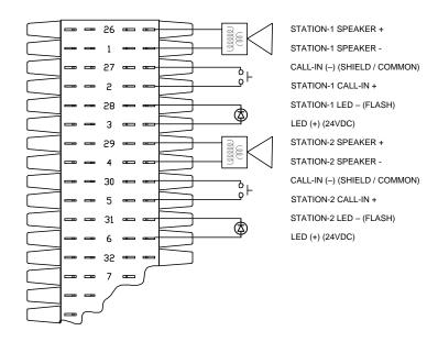
Punch blocks connect to the ICM via 25 pair cables with 50 pin connectors. Each group of 8 stations has its own 25 pair Amphenol connector that is laid out the same for station connections. So, if you have 16 stations there will be 2 of the 25 pair connectors and if you have 24 stations there will be 3 connectors and for 32 stations there will be 4 connectors.
