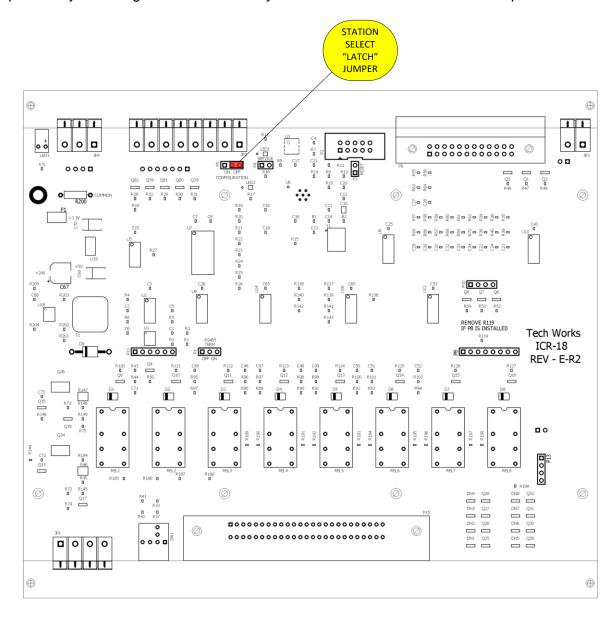
Diagram 1 Internal Latch / Hold Jumper
