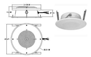
Tech Works Model CRS-RC complete, recessed mount loudspeaker system for hard ceiling applications in environments. clean room Rubber gaskets are included between the baffle mount screws and the baffle, the baffle and backbox, and between the backbox and the ceiling.
