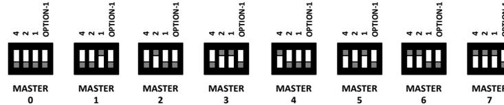
The dipswitch labeled "Column" is used to set the functional operation of the Zone Module. Each unit has the ability to monitor the first half of a single Master (Column 0-3), the second half of a Master (Column 4-7), a whole Master (all 8 columns), two whole Masters (the Master address +1), four whole Masters (the Master address +1, plus the Master address +2, plus the Master address +3), or All Master addresses. These functions are accomplished as follows.
