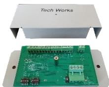
The Tech Works **CC2-CM-4** is an Intelligent Interface Module with screw terminals capable of supporting up to four passive push buttons and lights. The **CC2-CM-4** is a surface-mounting device constructed of cold rolled steel with a removable cover plate and is designed for use with normally open momentary contact closures.
