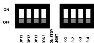
The Option dip switches S2 and S3 determine how each annunciator reacts to signals from remote stations. They also determine how and if the Annunciator sends messages to the network.
