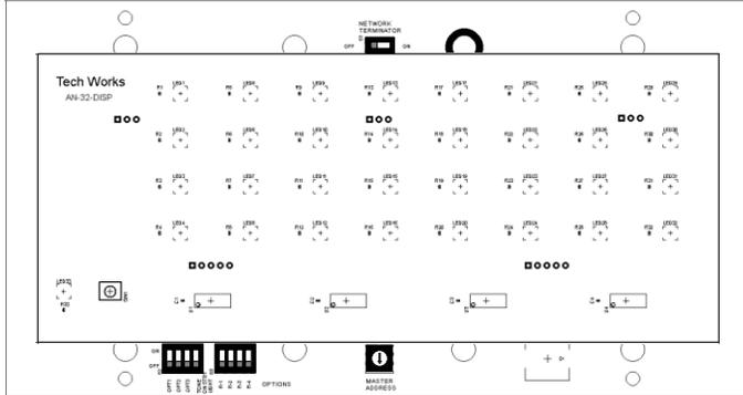
The **CC2-AN-84-T** has 8 columns of 4 lights. Each column corresponds to a CC2-RS-4 Room Status station, or a CC2-DL-44, or both at an Exam Room location. This is an 8 Exam Room annunciator with a built in Tone Unit.
