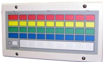
The Tech Works **CC2-AN-84-T** is an 8 Column, 4 Row, Lighted, Intelligent Annunciator panel. Made of white ABS plastic with a removable faceplate, each unit can be custom labeled to identify staff or locations. An integral tone sounds to draw attention to Emergency Calls. A big window allows for large labels of call points. Labels are back-lit so the call point lights up when a station is active.
