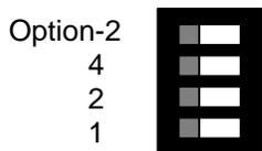
“Option-2” is the Flashing Light Tone On/Off switch
