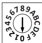
A rotary switch is provided for direct selection of the Master address to be monitored. Simply turn the arrow until it points at the Master address of the stations you want to display. Only the addresses 0-7 are active at this time in Clinic Call. Master addresses 8-F (16) are reserved for future expansion.
