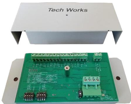
The CC2-CM-4 is an intelligent microprocessor based Dome Light station designed to work with our other Clinic-Call and Tech Works Network based products. Each CC2-CM-4 has 4 Contact Closure Switch inputs and a corresponding LED Light output.
