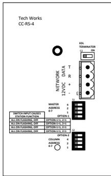
The **CC2-AN-4-T** is based on the same hardware as the CC2-RS-4 but includes a Tone unit and does not have any buttons to send signals. It addresses exactly the same as the CC2-RS-4 (see “Substation Addressing”) and is available in a variety of color options. The basic **CC2-AN-4-T** is designed to be a small 4 point annunciator for a single CC2-CM-4 or CC2-RS-4.
