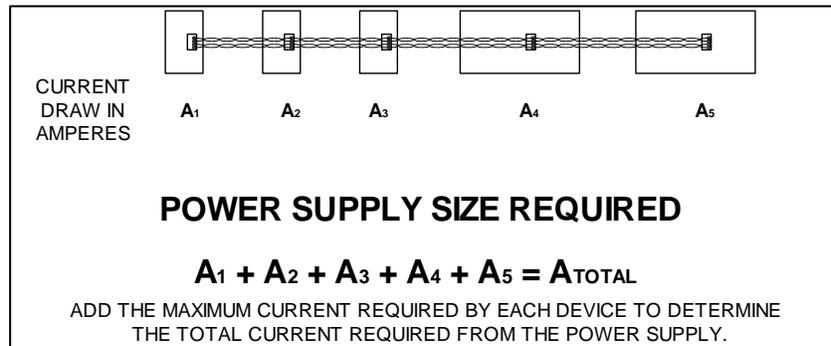
When system requirements exceed the current rating of a single power supply, then multiple power supplies can be used to support the system. Two rules apply to using multiple power supplies on a single Tech Works Network System:
