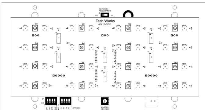
The **CC2-AN-16-T** and **CC2-MC-16-T** have 4 columns of 4 lights. Each column corresponds to a CC2-RS-4 Room Status station or a CC2-DL-44 or both at an Exam Room location. This is a 4 Exam Room annunciator with a built in Tone Unit.
