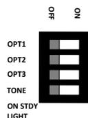
The OPT or Option switches determine how the annunciator responds to button pushes or signals from the network and what messages are sent to the network. The TONE Option switch turns on the function of a Tone associated with any Steady Lamp signal a Single Tone will sound with any Steady Light and a reminder Tone will sound every 20 seconds.
