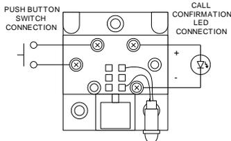
The HUBL Hold Up Button is a surface mounting plastic button with call confirmation light. The top snaps off to reveal the wire termination screws.
