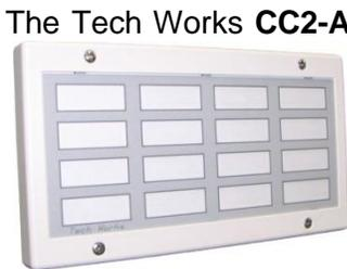
The Tech Works **CC2-AN-16-T** is a 16-Light Intelligent Annunciator panel. Made of white ABS plastic with a removable faceplate, each unit can be custom labeled to identify staff or locations. An integral tone sounds to draw attention to any change of status. A big window allows for large labeling of call points. Labels are back-lit so the call point lights up when a station is active.
