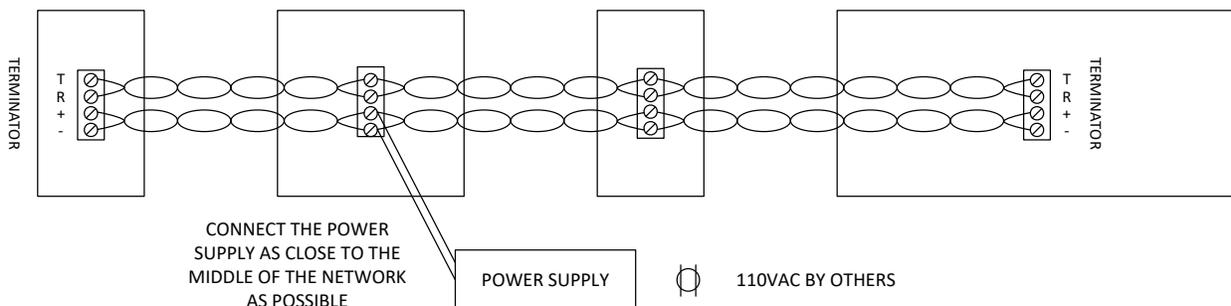
The system is designed to operate on unshielded twisted pair cable from 24 to 18 AWG. The twist of the cable is critical to the proper communication of data on the network to avoid noise interference. Any standard voice grade twist should provide adequate noise cancellation under normal operating conditions. All wiring is NEC Class 2.
