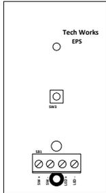
The EPS Emergency Pull Station is typically used in public Rest Rooms. It has a 36 inch pull string for easy access. The EPS also has a Push for Help button for those that prefer to push instead of pull for Help.
