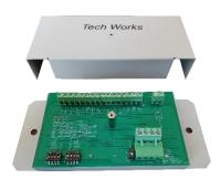
The Tech Works CC2-CM-4 is a mini Control Module designed to work with Tech Works Intelligent Networks. Units are equipped with screw terminals capable of supporting up to four passive push buttons and lights. The CC2-CM-4 is a surfacemounting device constructed of cold rolled steel with a removable cover plate and is designed for use with normally open momentary, or maintained, or normally closed maintained, contact closures.
