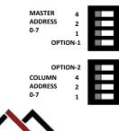
Each Substation is equipped with dipswitches for installer programming of the system. The first set of switches selects the Master or group of Masters on which this Substation will be displayed. The second set of dipswitches selects the column of lights on the Master to represent this Substation. Any two Substations with the same address will be totally interactive. This means the push of a button on one sub will light its light, as well as the light on the other sub with the same address.
