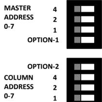
Each Substation is equipped with dipswitches for installer programming of the system. The first set of switches selects the Master or group of Masters on which this Substation will be displayed. The second set of dipswitches selects the column of lights on the Master to represent this Substation. Any two Substations with the same address will be totally interactive. This means the push of a button on one sub will light its light, as well as the light on the other sub with the same address.
