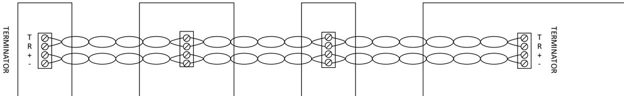
**Due to the implementation of innovative data noise canceling circuits in all Tech Works RS485 microprocessor products, the data and power can now be run in any direction up to a total wire length of 3000 feet.**
