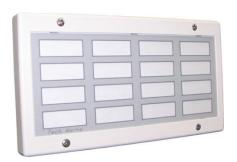
The Tech Works CC2-AN-16-T is a 16-Light Intelligent Annunciator panel. Made of white ABS plastic with a removable faceplate, each unit can be custom labeled to identify staff or locations. An integral tone sounds to draw attention to any change of status. A big window allows for large labels of call points. Labels are back-lit so the call point lights up when a station is active.
