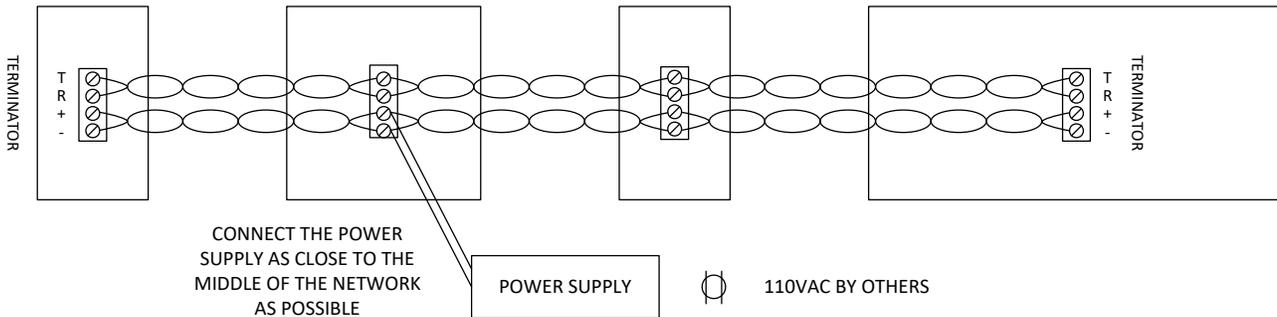
**Due to the implementation of innovative data noise canceling circuits in all Tech Works RS485 microprocessor products, the data and power can now be run in any direction up to a total wire length of 3000 feet.**
