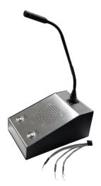
The DODC-1 includes a powder coated metal base with a stainless steel Faceplate, gooseneck condenser Microphone, a 3" Speaker, and 2 Vandal Resistant Push **Button Switches** specifically designed for the Detention industry. With its pre-wired cord it is perfect for those locations where some user control is required. The Face is Laser Engraved to prevent wear and destruction of labeling. One button is a "Talk" (Push To Talk) and the other is "Page".
