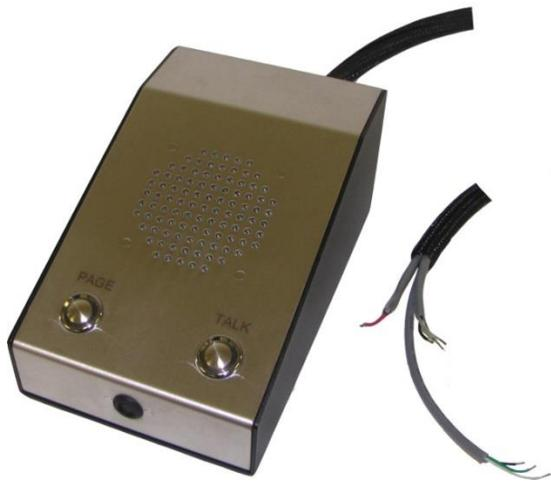
The DODC-2 includes a powder coated metal base with a stainless steel Faceplate, hidden condenser Microphone, a 3" Speaker, and 2 Vandal Resistant Push Button Switches specifically designed for the Detention industry. With its pre-wired cord it is perfect for those locations where some user control is required. The Face is Laser Engraved to prevent wear and destruction of labeling. One button is a "Talk" (Push To Talk) and the other is "Page".
