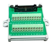
The Tech Works RC-BB-24 is a 24 pin Ribbon Cable Breakout Board designed to take our Tech Works 24 pin ribbon cables and make each conductor accessible by a screw terminal. These units are designed for the systems integrator and are typically used with our Intercom Relay products to allow fast easy installation with Programmable Logic Controls (PLC).
