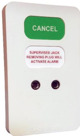
The Tech Works **NC-PBS-2** is a Dual Patient Bed Station in a semi-flush ABS plastic enclosure for durable emergency signaling. Two (2) ¼" phone jacks provide a supervised connection for a Call Cord like the **PBC-7**. The Call Cord provides the patient with call-for-help access when they may not be able to reach the station. Staff is provided with a distinctive "CANCEL" button to reset the station.
