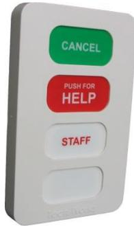
The Tech Works **NC-SPS** is a Staff Presence Station in a semi-flush ABS plastic enclosure for durable emergency signaling. A "STAFF" button generates a light signal to notify staff that someone is in a room. A convenient Push for Help button is also included for activating the Emergency Call directly at the station. Staff is provided with a distinctive "CANCEL" button to reset the station.
