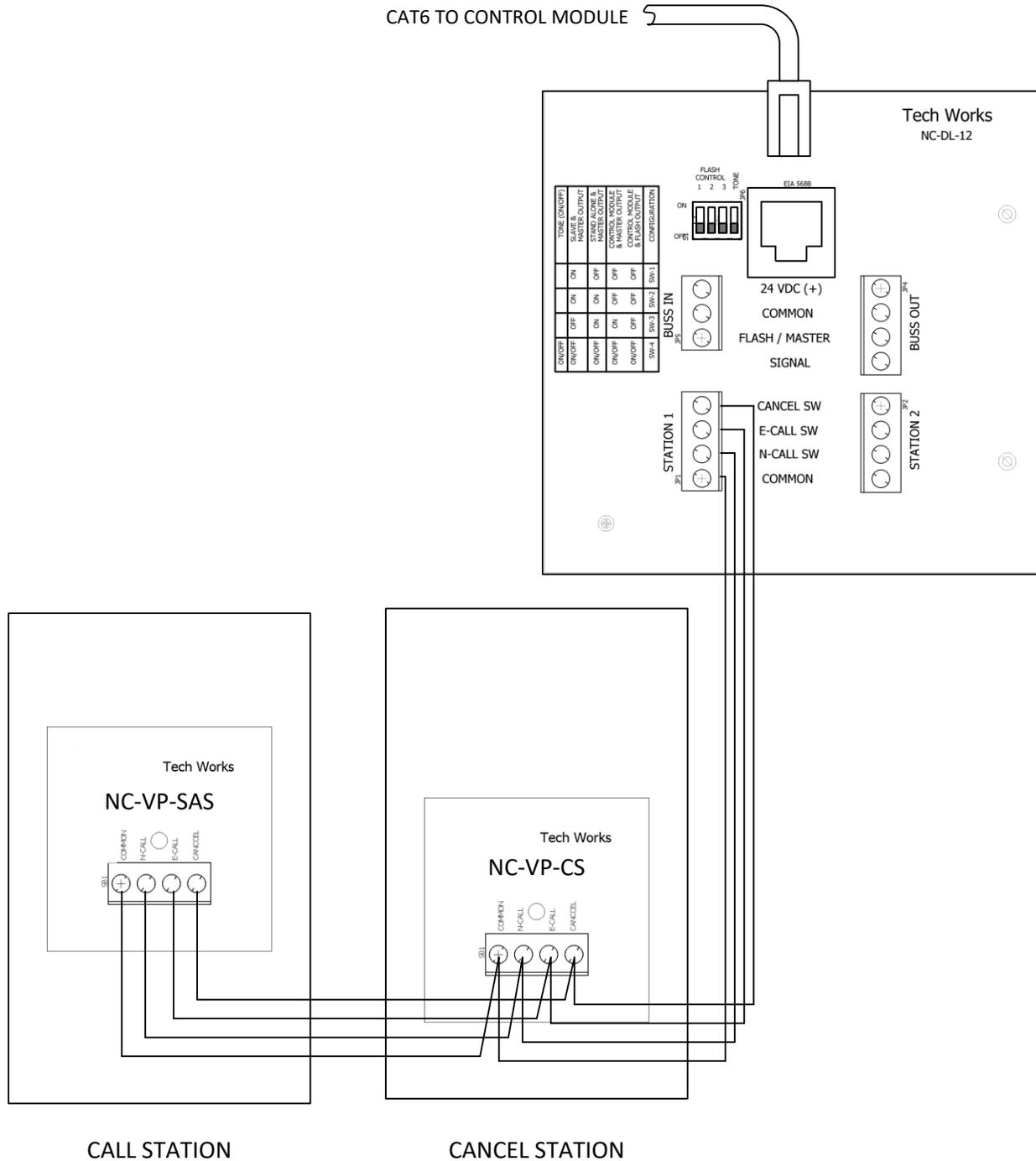
To install a Cancel Only Station simply hook it in parallel with and other Tech Works NC-Series Station
