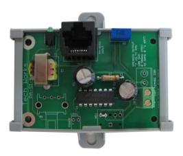
The **PA-SI-1** Speaker Interface is a 1-Watt Utility Audio Power Amplifier designed with the System Integrator in mind. The input is transformer balanced allowing several PA-SI-1's to be connected in tandem. Power comes from the PA-BUSS, to simplify wiring.
