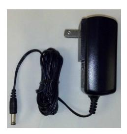
The Tech Works **PXX2410** is a regulated computer grade power supply capable of providing 1.0 Amp of power at 24-Volts DC to any of our products. This unit is UL and CSA listed in a wall mount enclosure. A 6foot power cord with a North American standard Edison connector is included. This is a switching power supply designed to operate on worldwide AC Voltage input.
