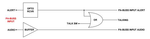
The CI-MSI-22 has an auxiliary audio input conforming to the PA-BUSS amplifier input. This input would normally be used for another Microphone input using the MHI-11, however any PA-BUSS output could also be accommodated.
