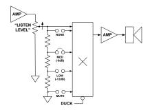
The Monitor/Communications level may be reduced to avoid Feedback, "Ducking". Ducking is invoked if:
