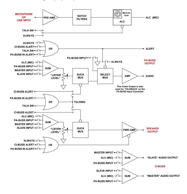
Simplified Block Diagram to illustrate some of the Configuration Jumper Options
