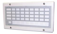
The Tech Works NC-AN-32C-T is a 32-Light Intelligent Annunciator panel. Made of white ABS plastic with a removable faceplate, each unit can be custom labeled to identify staff or locations. An integral tone sounds to draw attention to any change of status. A big window allows for large labels of call points. Labels are back lit so the call point lights up when a station is active.
