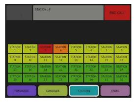
If a conversation is in progress with a remote and a second call is placed by another station, it will appear Red on the screen. In the case above, the console is talking to Station 4 while Station 3 is Calling In. All the other stations in this group of 16 are yellow indicting that they are unavailable. When the current Call with Station 4 is Ended the Yellow Icons will turn Green, the Call Tone will sound and any available operator can take the Call from Station 3.
