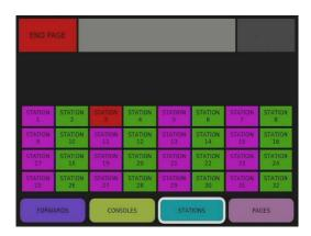
If another operator is paging and your console is in STATION screen you would see the current system activity. If a Call was active on the system that station would light up Red to indicate that a Call from station 3 will come in as soon as the Page is complete.
