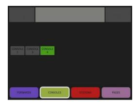
In the example this console is Operator #2 and is programmed to be able to contact Console 1, 3, and 4. However, Only Console #2 and #4 are currently connected to the system. To initiate a conversation with consoles #4, select the Icon and the following screen appears. If console #4 accepts the call by answering it the operators can speak to each other just like talking to a remote.
