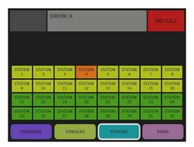
The screen will change to look like this. Only one console can talk to a station in a group of 16 remote stations at a time. When a group of 16 station is "Busy", they will turn Yellow on all Operator consoles to tell everyone that a conversation is in progress. The remote station engaged in the conversation will turn Orange to indicate that it is talking to an Operator.
