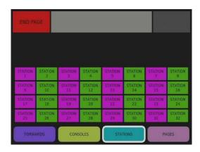
If at any time the operator wants to see exactly which stations are selected for a page, they can select "STATIONS" while the page is active and the stations to be addressed will be hi-lighted in Purple.
