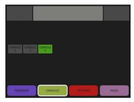
If your console is in a different screen and there is a call pending on the system, the STATION button will turn Red telling the Operator to press the STATION button to see and answer the pending call.
