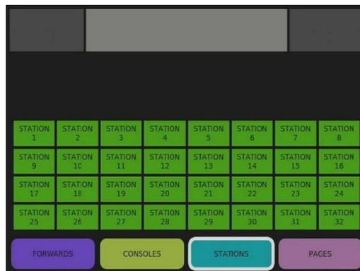
This screen shows that 32 stations are connected and programmed to call this ODC.
