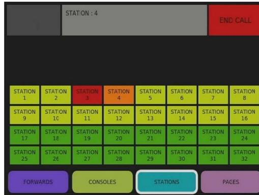
If a conversation is in progress with a remote and a second call is placed by another station, it will appear Red on the screen. In the case above, the console is talking to Station 4 while Station 3 is Calling In. All the other stations in this group of 16 are yellow indicating that they are unavailable. When the current Call with Station 4 is Ended the Yellow Icons will turn Green, the Call Tone will sound and any available operator can take the Call from Station 3.
