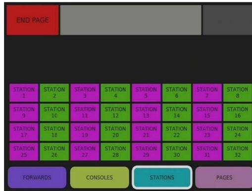
If at any time the operator wants to see exactly which stations are selected for a page, they can select “STATIONS” while the page is active and the stations to be addressed will be hi-lighted in Purple.
