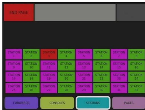
If another operator is paging and your console is in STATION screen you would see the current system activity. If a Call was active on the system that station would light up Red to indicate that a Call from station 3 will come in as soon as the Page is complete.
