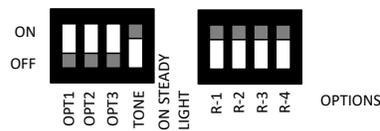
Dip Switches are used to set the software Options in the NC-AN-16C & 32C-T Annunciators. The switches shown are in the Default position. All Dip Switches are OFF when down and ON when up. The switches labeled “OPT1”, “OPT2”, and “OPT3” are not active in the NC-AN-16C & 32C-T Annunciators. These are reserved for the Clinic-Call Annunciator products.
