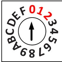
The Address switch is only read when the processor is rebooted. To have any change of address take effect the power must be cycled so that the address switch will be read.
