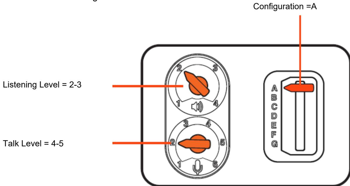
If your system uses a microphone and speaker in conjunction with your headset, be sure to adjust the microphone and speaker for proper listening levels, per their product manual, before adjusting the headset levels. Then adjust the headset levels to best match the levels of the console microphone and speaker.
