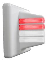
The MC-NC2-DL-22-RW is a stylish, exceptionally bright Nurse Call Dome Light. It is the central tie point for the Patient Room, with wiring going to the Call Stations and to the Central Control Module. The Call stations are equipped with Momentary Switches that are monitored and latched in the Central Control Module. The Call stations have Call Confirmation Indicators that display the same output as the Dome Light.
