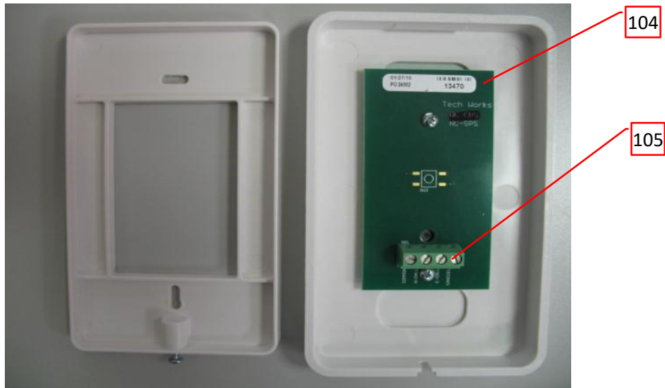
Photo 39 - Nurse Call Code Blue plus Assist Station NC-CBAS - Back View - PCB - Side 1
