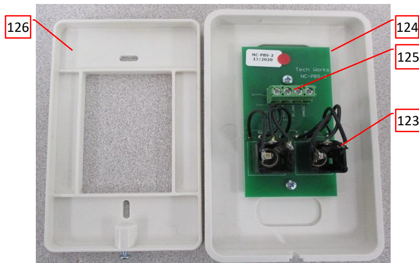
Photo 48 - Patient Bed Station Model NC-PBS-2 - with 2 call jacks - PCB
