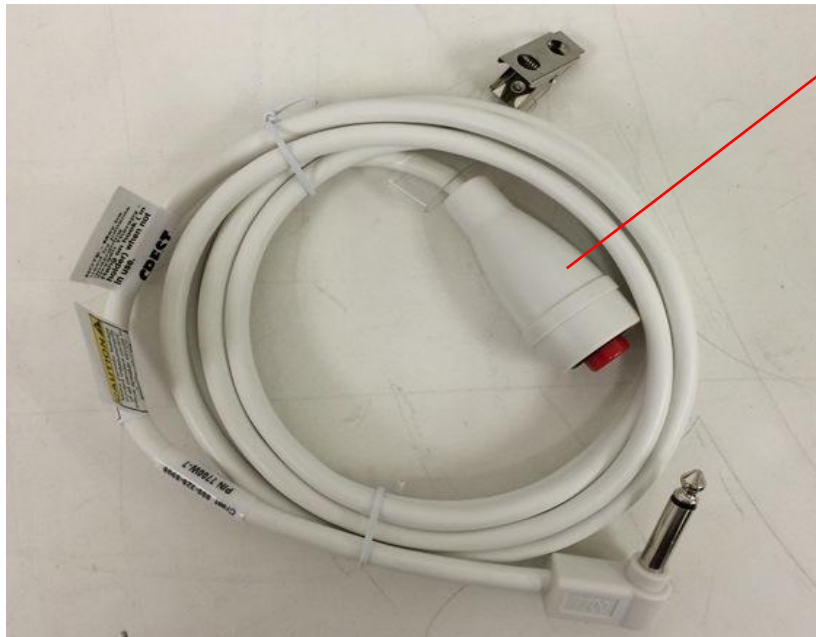
Photo 9 - Push Button Call Cord Model PBC-7 (Used in conjunction with Emergency Push Button Station Model NC-PBS-1)
